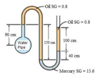
(b) Find the specific gravity, SG<sub>2</sub> for the following manometer.
